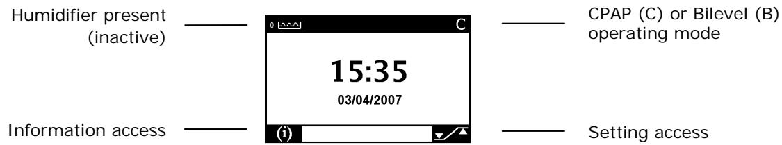
**Figure 2 – View of display in standby mode**
