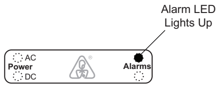
Figure 7–3 Alarm LED Lights Up
