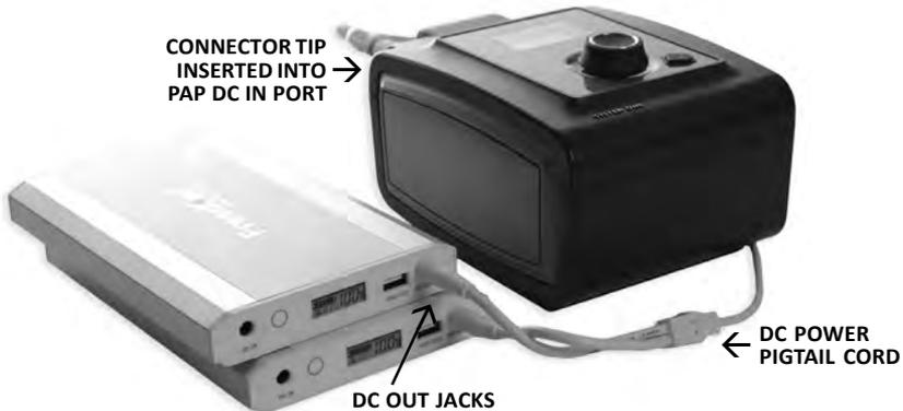
Image shows connection to Respironics System One 60 series PAP device.
