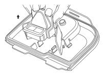
2. Remove the baffle (2) by pressing in on the side tabs and pulling up on the baffle.
