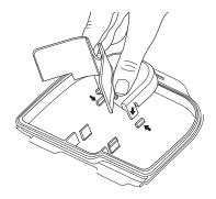
6. Reassemble the manifold. Align the manifold with the hooks on the tank lid. Gently press down on both manifold blocks until they snap into place.
