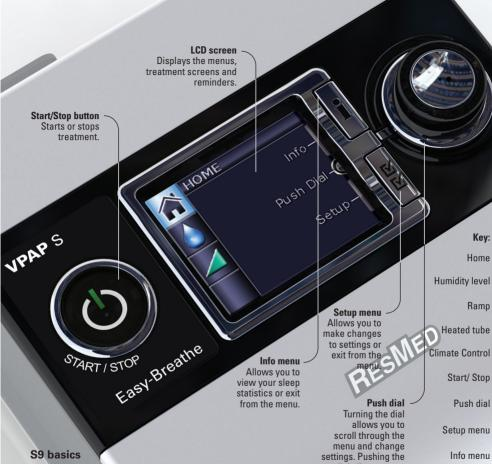
The control panel of your S9 device includes an LCD screen as well as a Start/Stop button, Push dial and the Info and Setup menu keys.
