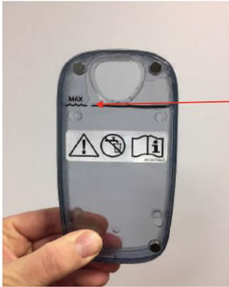
Reservoir should be filled to the 'Max Fill' line.
